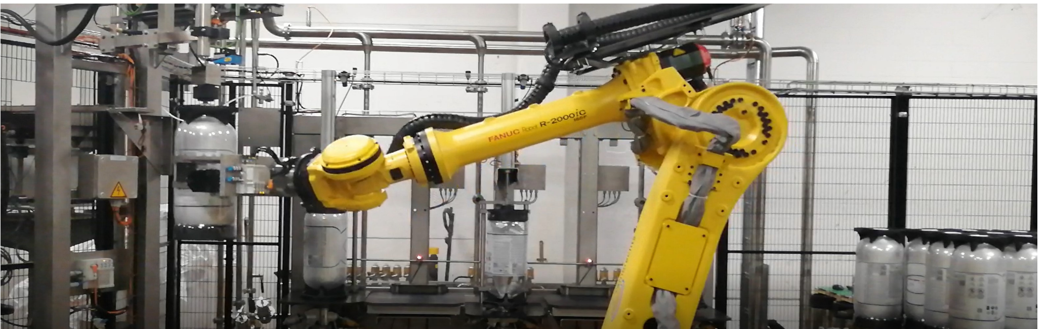
High capacity one way keg filling, capping, collar application and palletizing with robot
